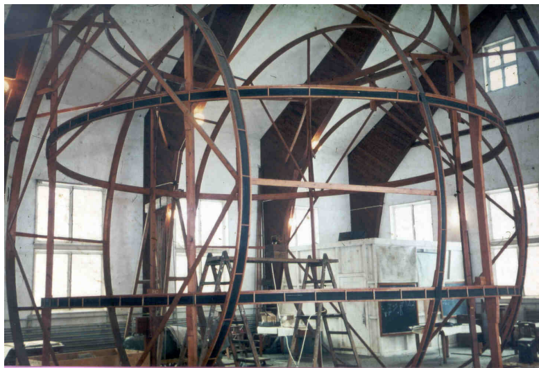
Wingst Observatory: Fanselau coil system constructed in 1943
