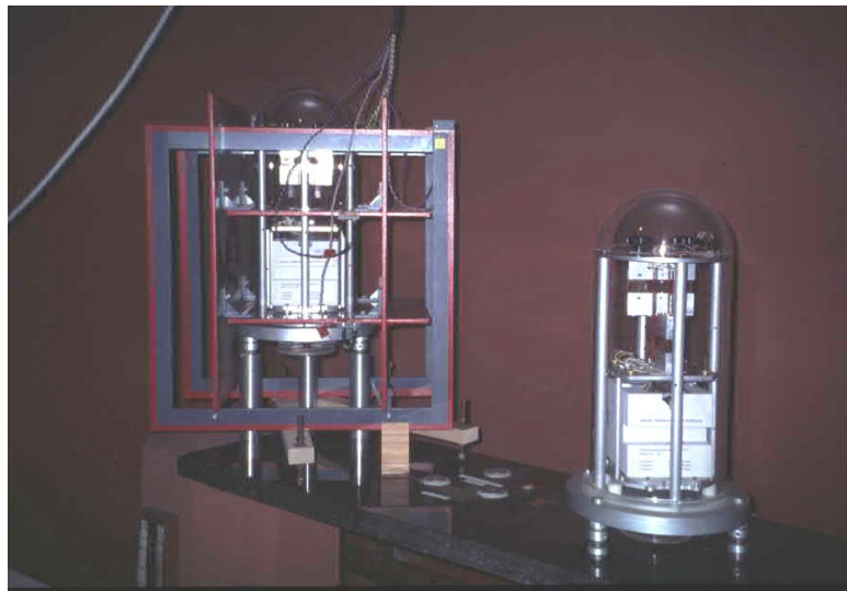
FGE double system at Wingst Observatory. One of the suspended triples is provided with a coil system constructed after Beblo et al. (1999)
